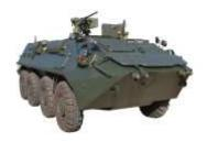
Amphibious armored personnel carrier **SAUR-2** 8x8 type is homologated by Romanian Ministry of Defense. The vehicle is designed with protection level 2, 2a and 2b, in accordance with STANAG 4569, with diesel engine and automatic gearbox.
